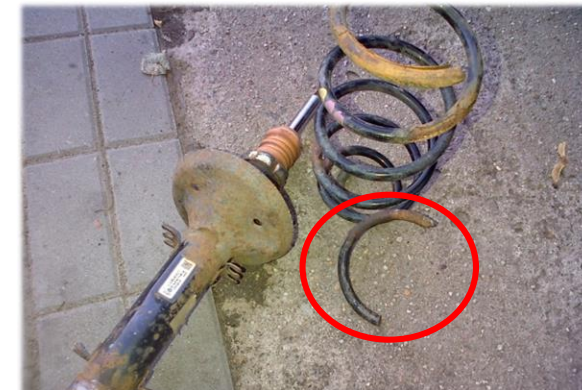
Broken suspension spring exchange (Octavia I)
