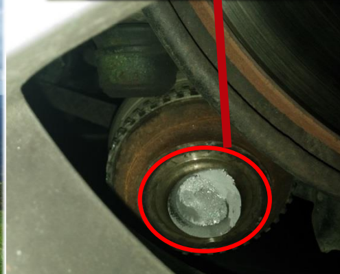
Twisted Rear wheel half axle ( Mazda MX-5)
