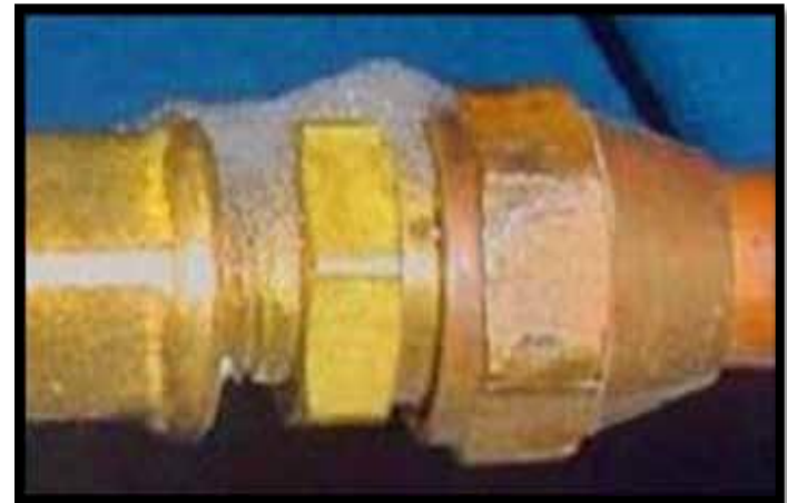
Foam film and bubbles to detect gas[1]
