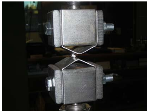
Fig 2.3: Failure of spot welded coupon for pure tensile loading condition [7]
