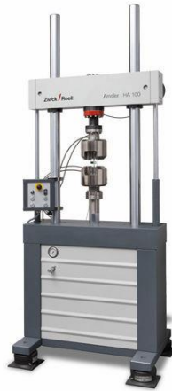
Fig.4.5. Schematic of acoustic emission resonant tensile fatigue setup
