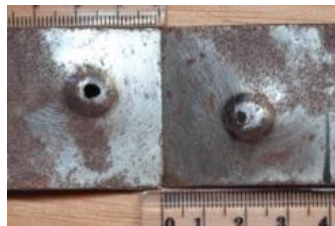
pullout failure (PF) mode
