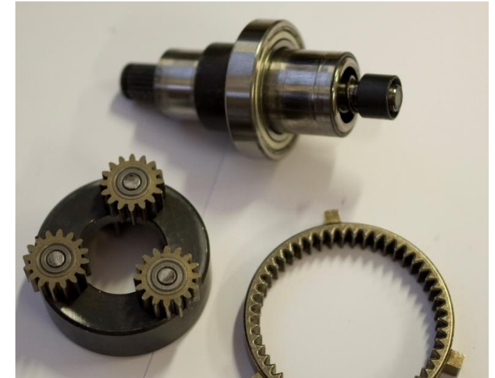
6KT - Planetary gear of starter (Magnetron)
