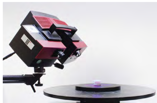
Figure 1. Measuring by ATOS III Triple Scan 3D optical scanner.
