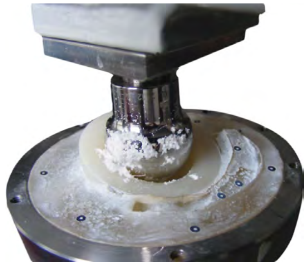
Figure 8. Validation test by hip pendulum.
