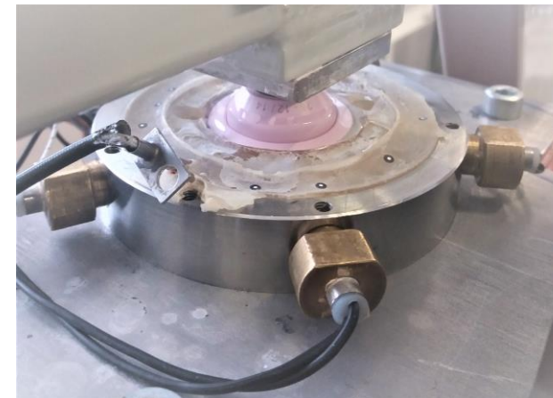
Ball-on-cup Configuration within hip joint simulator
