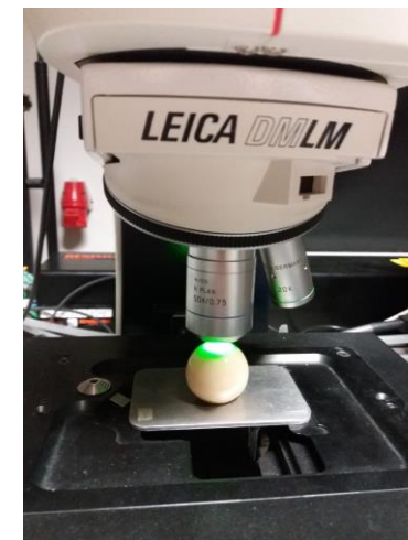
Raman Spectroscopic measurements for BIOLOX®forte implant surfaces with SF Lubricant
