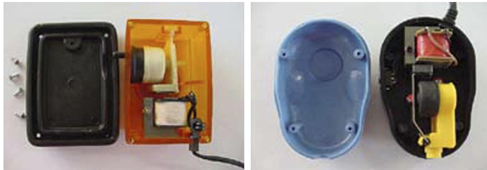
Fig. 2-10 Internal design of compressors for aquariums [9].
