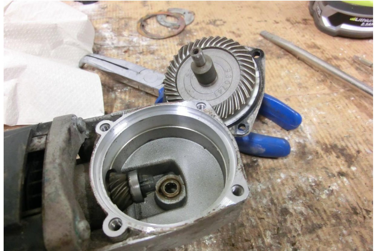
Gearbox of Angle Grinder - Missing lubricant
