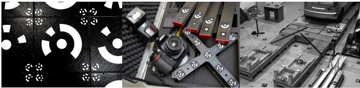
Figure 2. On the left – hybrid calibration targets, in the middle – TRITOP (GOM) measuring system with GOM CFK scale bars, on the right – an example of large calibration field.
