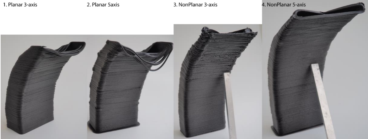
Figure 30 Comparison of different multiaxis 3DP methods: Planar 3 axis, Planar 5 axis Oriented, Nonplanar 3 axis, Nonplanar 5 axis Oriented
