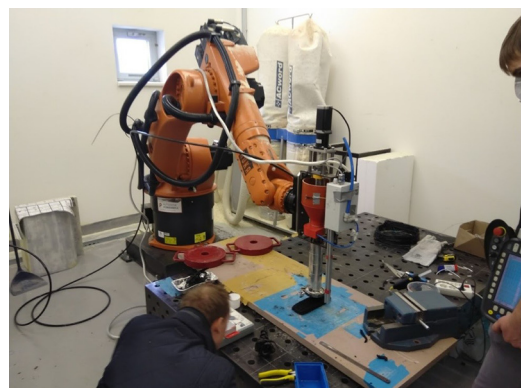
Figure 2 Single screw extruder mounted on KUKA robot arm, shown during a test print
