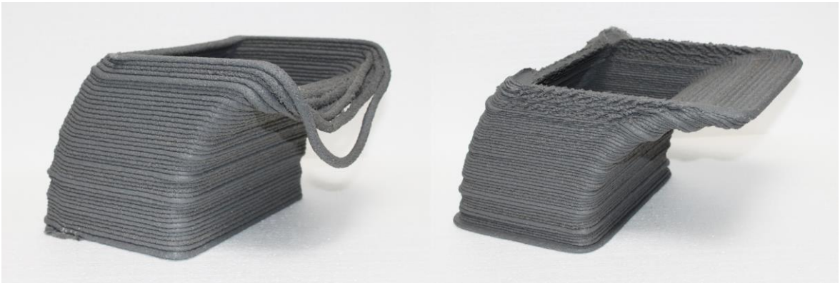
Figure 36 Buildability extension by the intralayer height variation method Left - 3-axis Right - Intralayer variation
