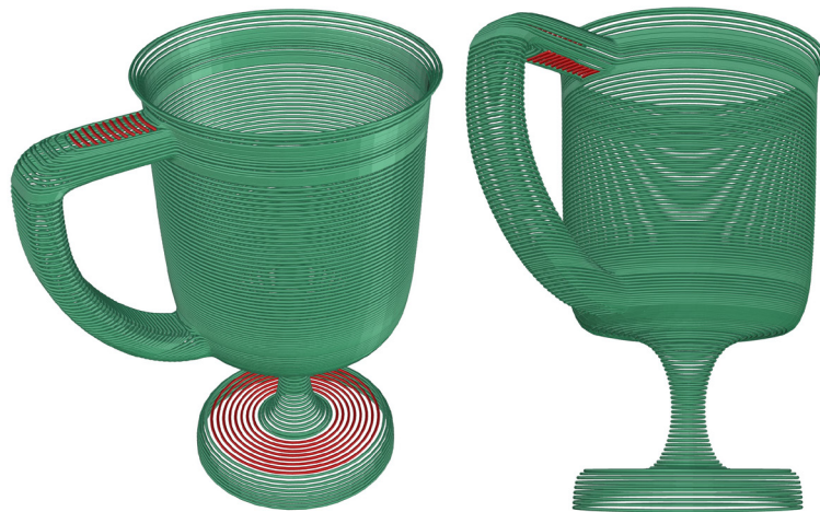
FIG. 14. Sliced glass with zones to be printed with 2D slicing marked in black ; toolpaths are thickened for visibility. 2D, two-dimensional.
