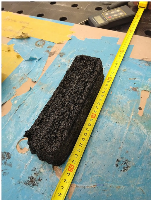
Figure 6 Longitudinal sample after printing, still on its print surface
