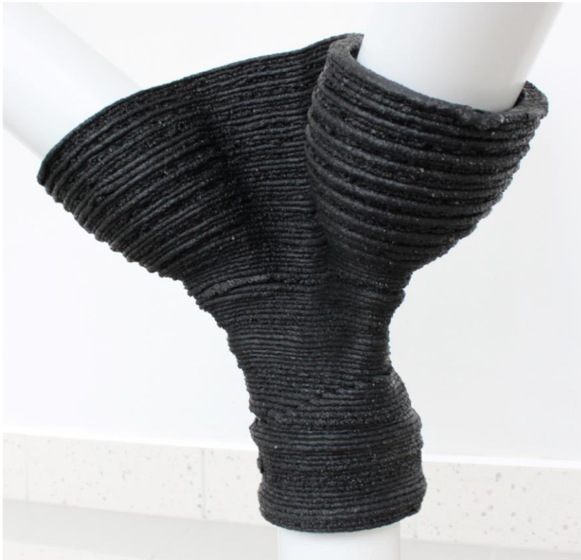
Figure 2 Beam joint printed using polymer concrete and nonplanar toolpaths for a conference submission
