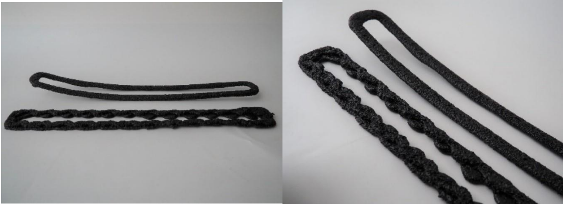
Figure 28 Effect of print path modification on warpage of polymer concrete deposition
