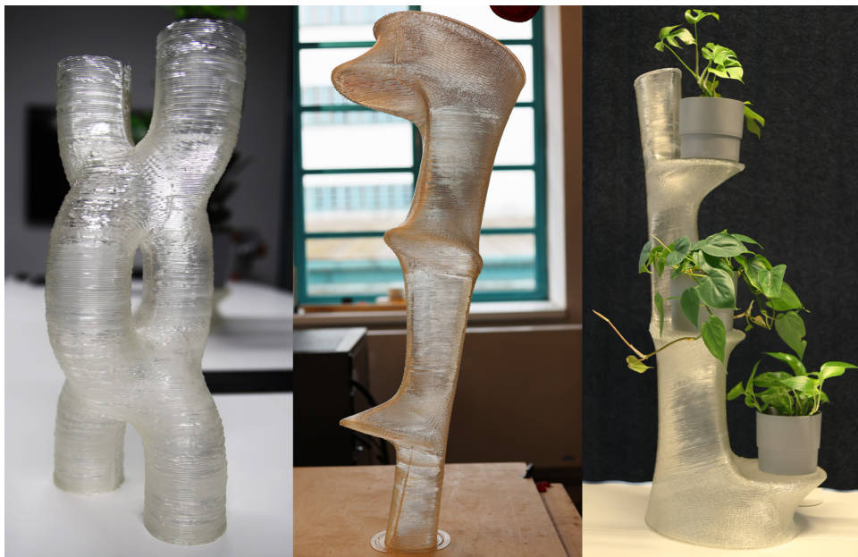
FIG. 15. Left : The chain link sample sliced and printed with the described method (Leftovers after retractions removed). Right : Flower planter stand printed with the described method, as printed and in use.
