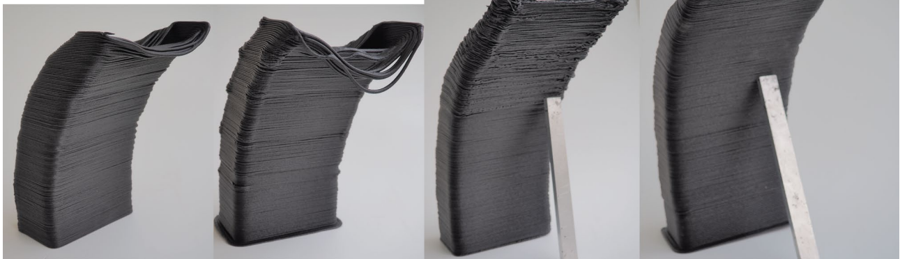
Fig. 11 All the prints side by side, from left to right: planar 3-axis, planar 5-axis, nonplanar 3-axis, nonplanar 5-axis
