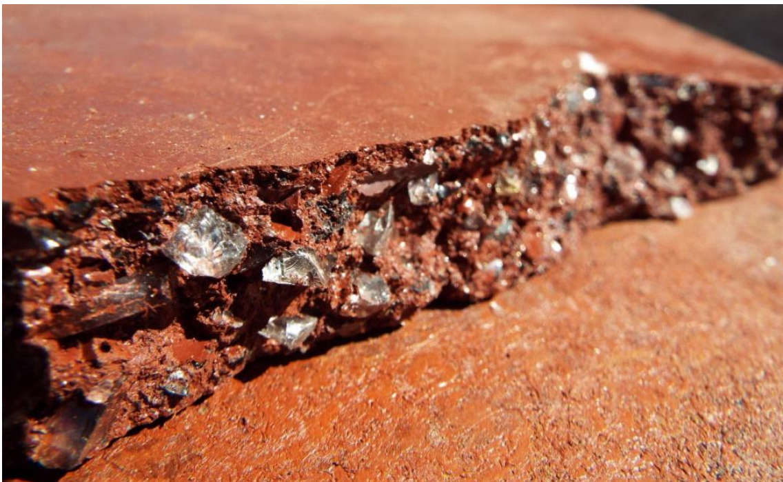
Figure 1 A tile cast from a polymer concrete mixture based on post-consumer PET and reclaimed glass [5]
