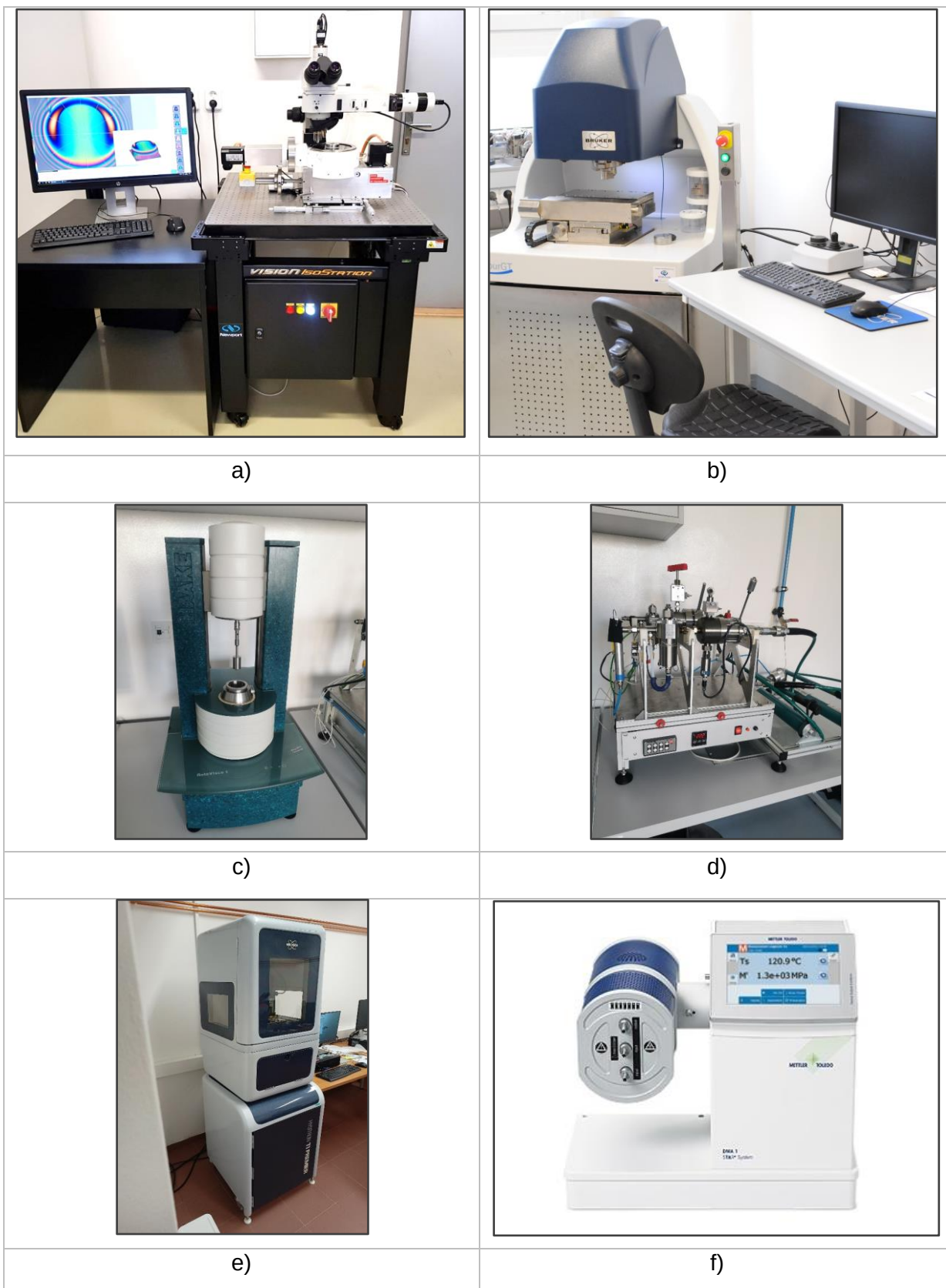
Fig. 30. Experimental equipment used. a) rotary optical tribometer (Brno University of Technology, Czech Republic), b) Bruker 3D optical profilometer (Bruker, USA), c) HAAKE RotoVisco1® (Thermo Fisher Scientific, USA), d) HPV (Brno University of Technology, Czech Republic), e) Hysitron TI Premier Nanoindenter (Bruker, USA), f) DMA1 (Mettler Toledo, Switzerland).
