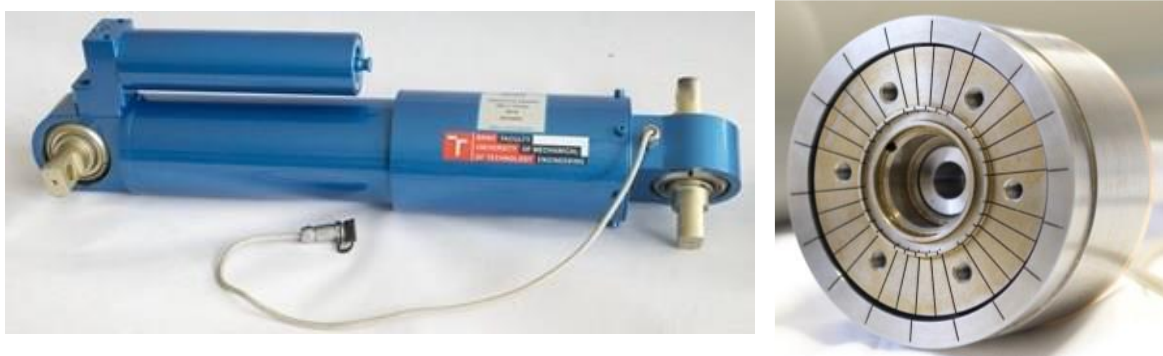
Fig. 7-1 MR damper for railway vehicle application (left) and its grooved magnetic circuit (right) [108]
