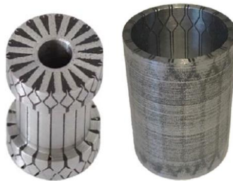
Fig. 2-34 Structured core and outer cylinder of MR damper valve made by SLM [59]
