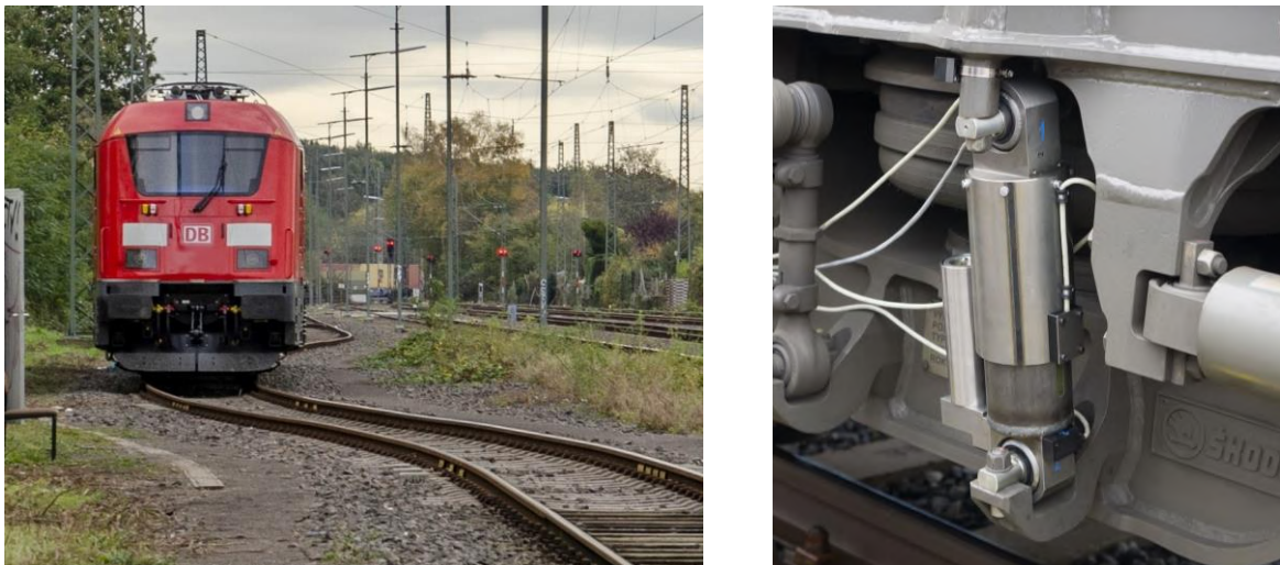
Fig. 7-3 Running test (left); mounting of the MR damper to railway vehicle (right)
