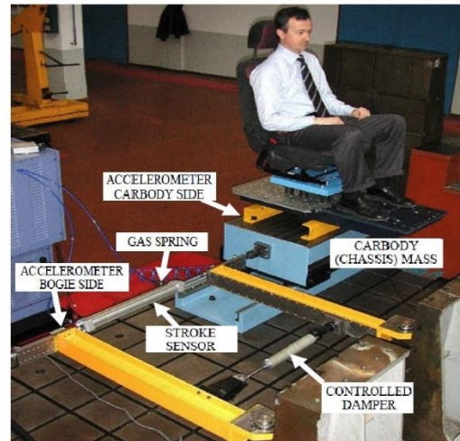
Fig. 2-21 Test-bench of carbody lateral movement [7]
