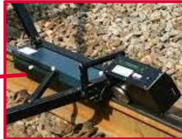
Hand-pushed tribometer (www.lbfoster-salientsystems.com)
