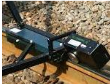
Hand-pushed tribometer (www.lbfoster-salientsystems.com)
