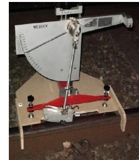
Pendulum tribometer (Lewis, S.R., 2011)
