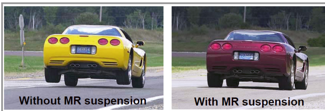
Obr. 1.11 Systému Magnetic Selective Ride Control na modelu Chevrolet Corvette C5 [22]
