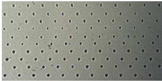
Fig. 5.7 Microscopic image of dented ball surface by Rockwell indenter.
