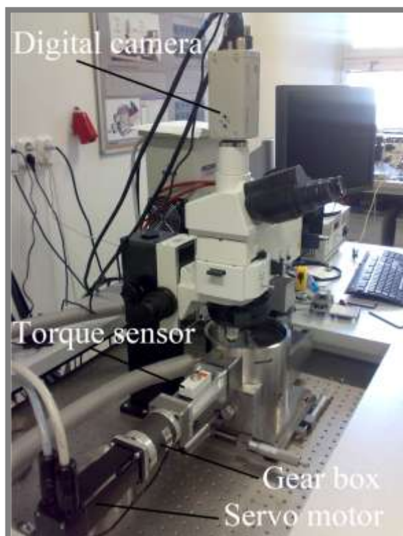
Fig. 25 Tribometer equipped by a torque sensor and a digital camera
